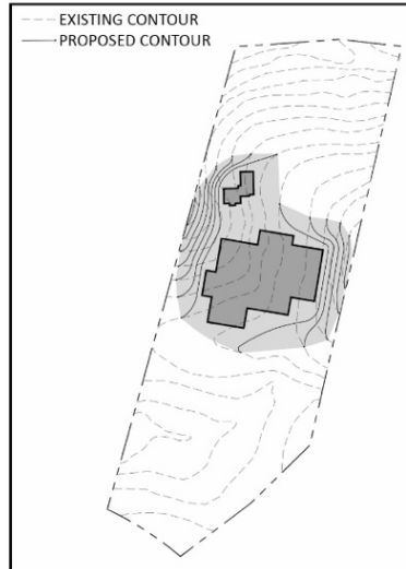
BUILDINGS PERPENDICULAR TO CONTOURS (Requires more grading and requires less desirable contour grading)
